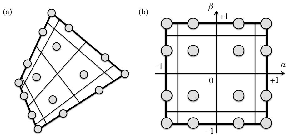
FIG. 6: (a) Artificial control volumes associated with degrees of freedom in a fourth-order Gauss-Lobatto-Legendre finite element and associated GLL quadrature nodes. (b) Artificial control volumes in the fourth-order Gauss-Lobatto-Legendre reference element and associated GLL quadrature nodes, with coordinate axes  $\alpha \in [-1, 1]$  and  $\beta \in [-1, 1]$ .
