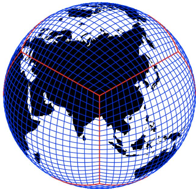
Third-order finite-volume method on the cubed-sphere grid. Accuracy drops to second-order due to dimension splitting.
