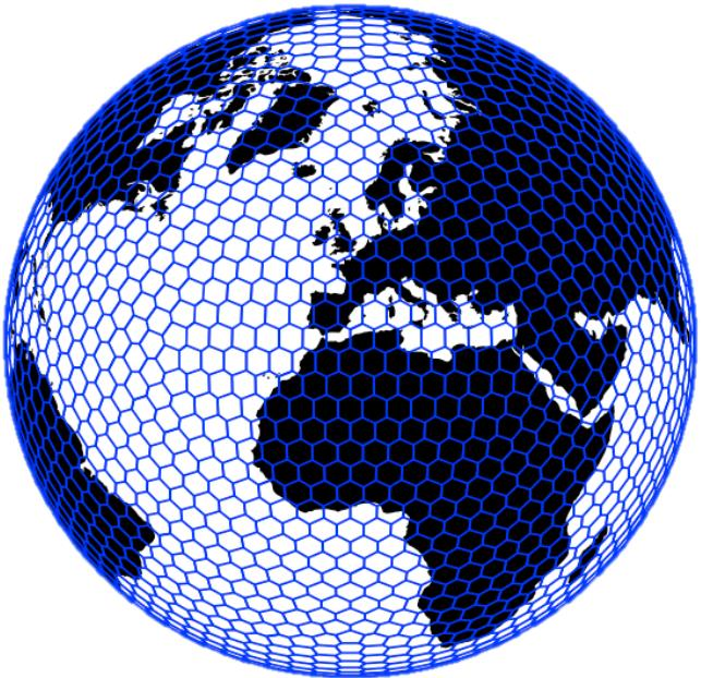
The model is based a hexagonal grid which has been optimized via a post-processing step.
