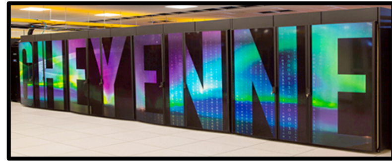
NCAR Cheyenne supercomputer (5.34-petaflops in 145,152 cores)
