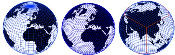
Figure 4: Left: A latitude-longitude mesh. Center: An icosahedral (geodesic) mesh. Right: A cubed-sphere mesh.
