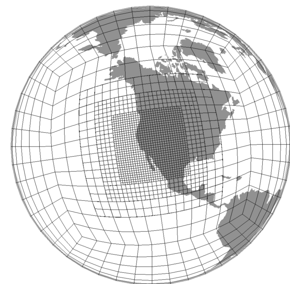
Figure: A non-conformal block-refined mesh with three levels of mesh refinement over California.
